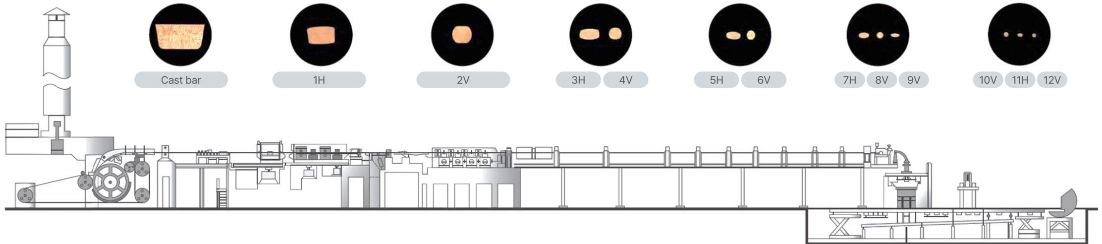
Melting → Casting → Rolling → Pickling & Coating → Coiling & Coil Handling
